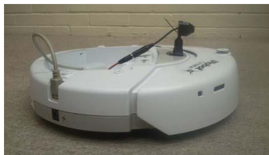
Figure 4: Picture of a Roomba Create mounted with a wireless camera.
