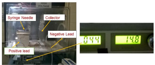
Figure 3: Experimental setup of electrospinning process for the production of the PCL nanofibers.
