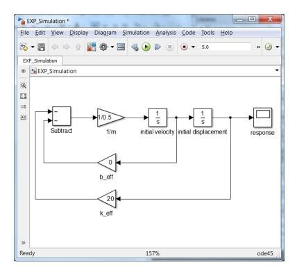
Figure 5 A schematic of Simulink module
