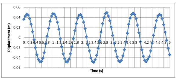
Figure 4 An experimental response of the 2nd order spring-mass system
