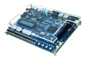
Figure 1: DE2-115 FPGA development board used in this course.
