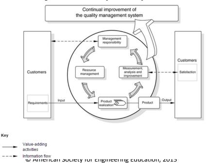
Figure 1. ISO 9001-2008 Continuous Improvement Process<sup>11</sup>
