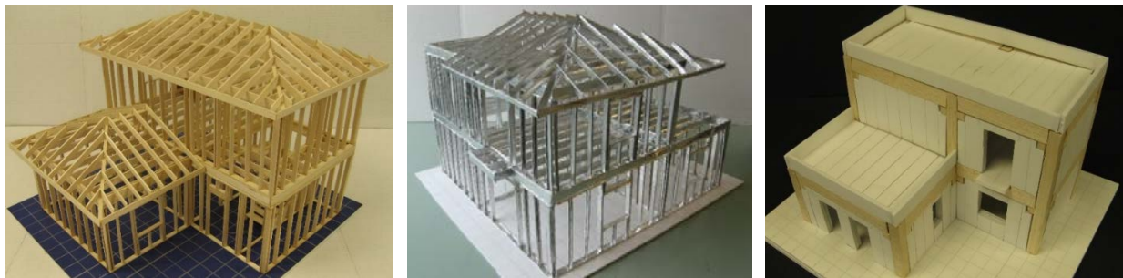
Figure 8. General overview of timber and CFS framing models in 1/20 scale and RC prefabricated model in 1/32 scale
