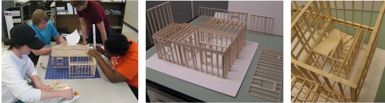
Figure 5. Assembly of timber framing model in 1/20 scale
