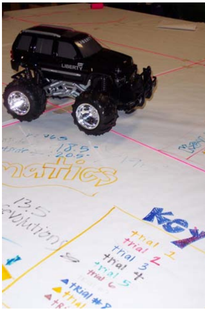
Figure 8. RC model Jeep Liberty SUV performing a non-incremental Lie bracket maneuver.
