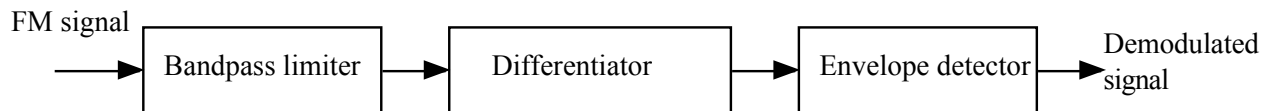
Figure 4: The block diagram that describes FM detection in a typical communication systems textbook.
