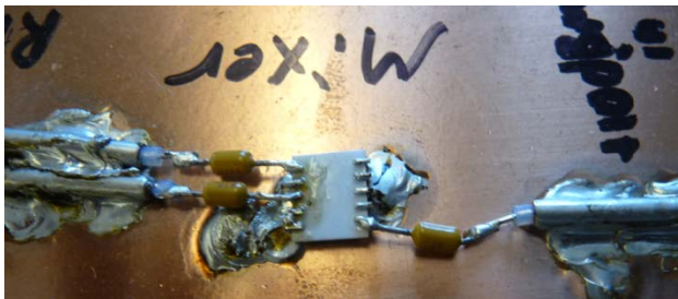
Figure 4: This figure shows a surface-mount mixer connected to the 0.085 inch semi-rigid coaxial assemblies. The surface mount mixer has several pins that are grounded to the PC board in order to hold the mixer solidly in place. Next the semi-rigid coax is put into place. Finally, the radial lead capacitors are used to interconnect the coax to the mixer. The solder quality on the right is adequate, while the left side is marginal.
