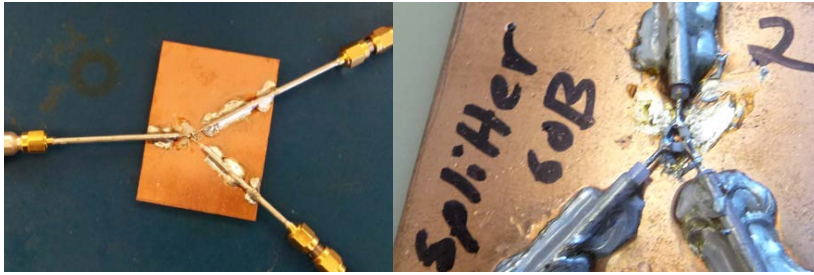
Figure 3: The picture on the left shows a three-resistor power splitter along with the three 0.085 inch semi-rigid cable assemblies constructed by the class. The figure on the right shows a close in photo of the three-resistor splitter. The three resistors are each 16.66 ohms giving each port a 50 Ohm impedance and 6 dB nominal signal loss. This assembly project is challenging for the students and requires proficiency in handling and soldering small parts. The center conductor lead length is minimized so that the inductance does not limit the frequency performance of the splitter. The students learn the importance of circuit miniaturization as a result of building these components.
