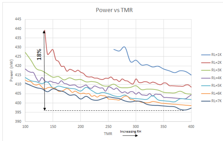
Figure 4. Observing power dissipated in the circuit as a function of increasing TMR for various constant low resistances (RL)
