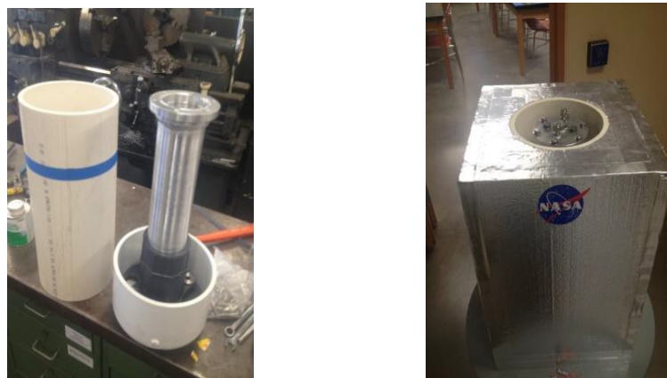
Figure 14. CO 2 Cryogenic Separator on PVC Base (left); styrofoam insulated housing (right).
