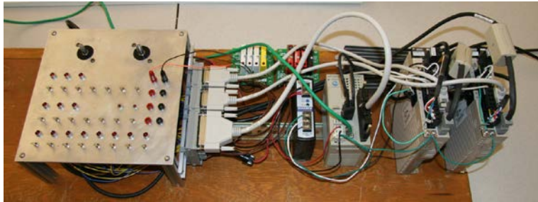
Figure 3. Yaskawa 2-Axis servo-motor control trainer.
