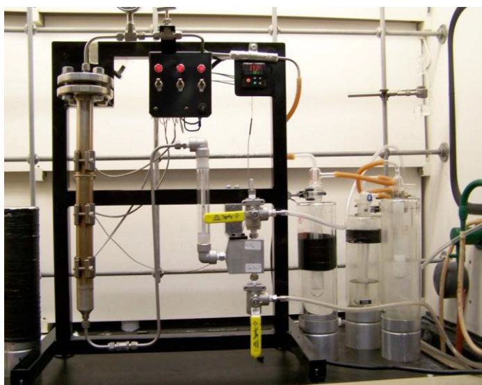
Figure 3. Table-top Sabatier reactor with cryogenic separation dewars.
