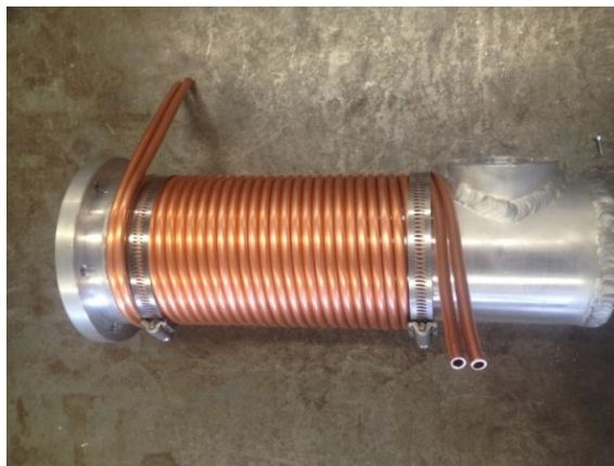
Figure 13. Water cryogenic separator with copper cooling coils.
