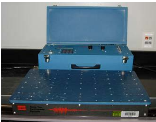
Figure 3. Small shake table (single-axial excitation).
