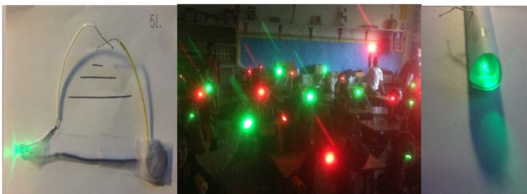
Figure 2. Students study the conductivity of graphite, calculate the ratios between lengths of the graphite lines and compare with the brightness of the LED, and roll-up their note card to build a simple flashlight.
