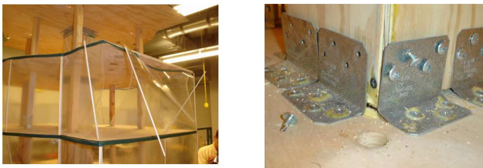
Figure 19. Non-structural and structural failures occurred during testing without damper.
