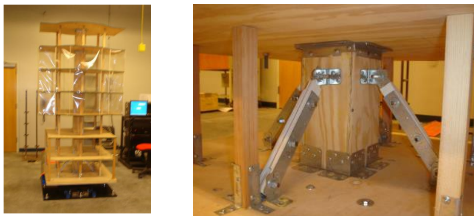
Figure 18. Multi-story housing structure with friction damper at the base level.
