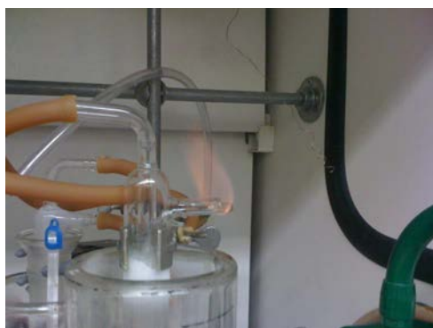
Figure 5. \text{CH}_4 flame at output.
