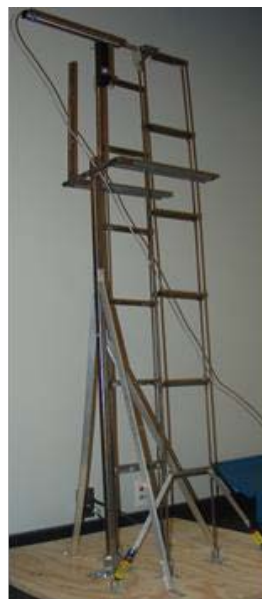
Figure 5. Linear displacement sensor used to measure story drift.
